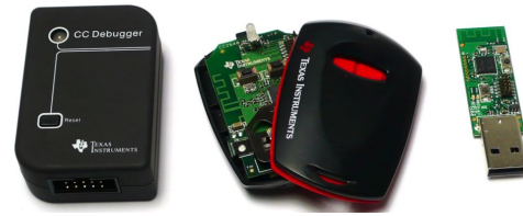
Figure 2. Texas Instruments CC2540 Mini Development Kit includes, from left to right, a debugger for programming BLE devices, a key fob BLE device, and a USB dongle BLE device.
