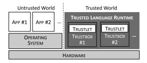
Figure 1: High-level architecture of TLR.
