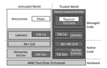
Figure 2: Component diagram of the entire system with a TLR: the darkest shade shows the TLR components, the light gray shows the smartphone's standard system components, and the application components are in white.
