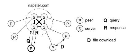
Figure 2.4: The architecture of Napster. Peers send their queries to the Napster central cluster of servers, in a client-server manner. Files are transferred among peers, in a peer-to-peer manner.
