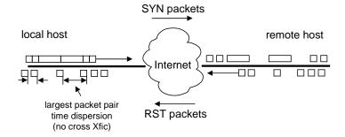
Figure 3.6: The consistent arrival times heuristic test. The time dispersion of the RST packets corresponding to the large SYN packet pair (the middle packets) should be the largest dispersion among packet pairs when no cross traffic is present.
