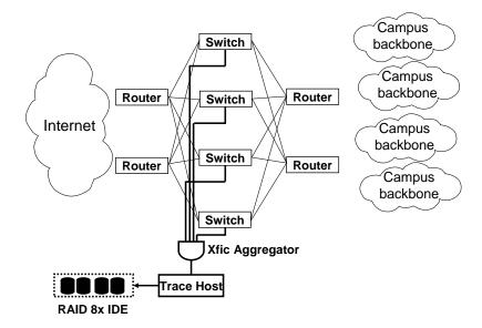
Figure 3.1: The integration of our network tracing system within the University of Washington network border configuration.
