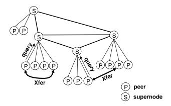
Figure 2.7: The architecture of Kazaa. Each peer is connected to exactly one supernode. Supernodes form an overlay network. Files are transferred among peers.
