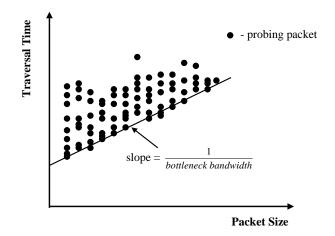
Figure 6.1: One-Packet Model: ideally, the minimum value of the traversal times for each packet size approximates a line whose slope is the inverse of the bottleneck bandwidth.
