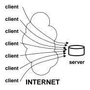
Figure 2.1: The layout of a Web client-server architecture on the Internet.
