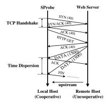
Figure 3.7: The packet exchange initiated by SProbe to estimate the bottleneck bandwidth in the upstream direction.
