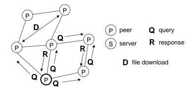
Figure 2.5: The architecture of Gnutella. Peers form an overlay over which queries are flooded. Files are transferred among peers.
