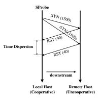
Figure 3.5: The packet exchange initiated by SProbe to estimate the bottleneck bandwidth in the downstream direction.
