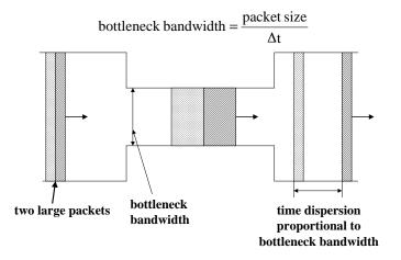
Figure 6.2: Packet Pair Model: after the bottleneck link, the time dispersion between the packets is proportional to the bottleneck bandwidth.
