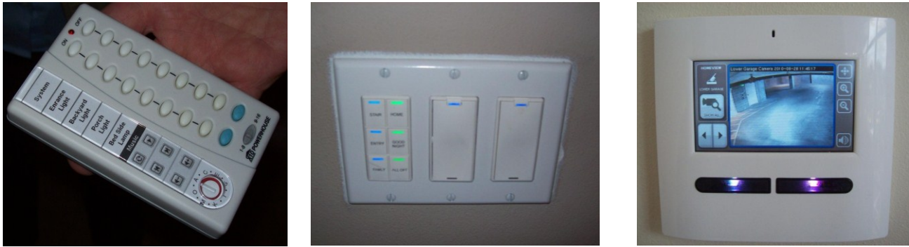
Figure 1: Home Automation User Interfaces: remote control for lighting scenes (left), augmented light switches (center), wall panel with remote camera view (right).
